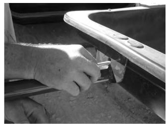
**Step 9:** Before raising the Horse Rack Brace (HRBH) vertical, insert a carriage bolt (3/8" x 2 ½") (FB062.50ZPG2) through the saddle from the side facing outward. (See fig. 8)
