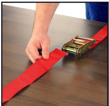
1) Insert loose end of strap into mandrel of ratchet
