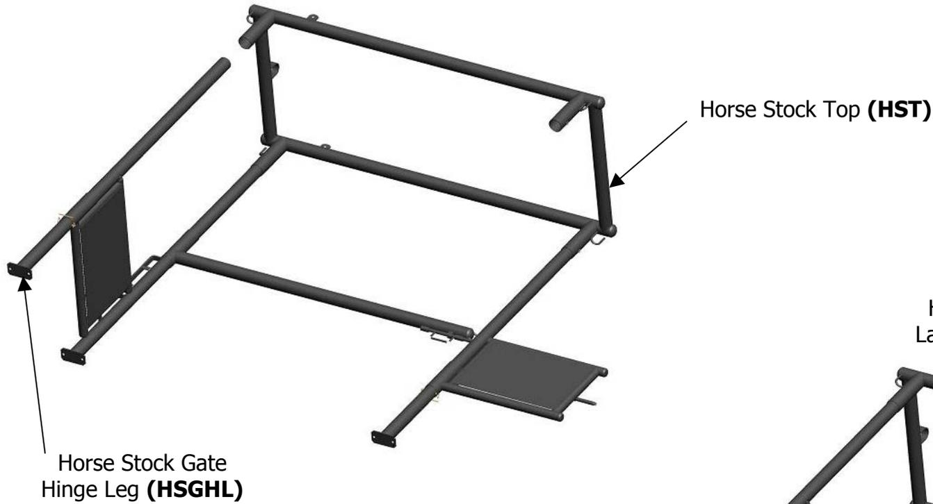
**Step 6:** Insert the other (HSGHL) into the (HST) and secure it with the 3/8"X3/4" Set Screws provided.
