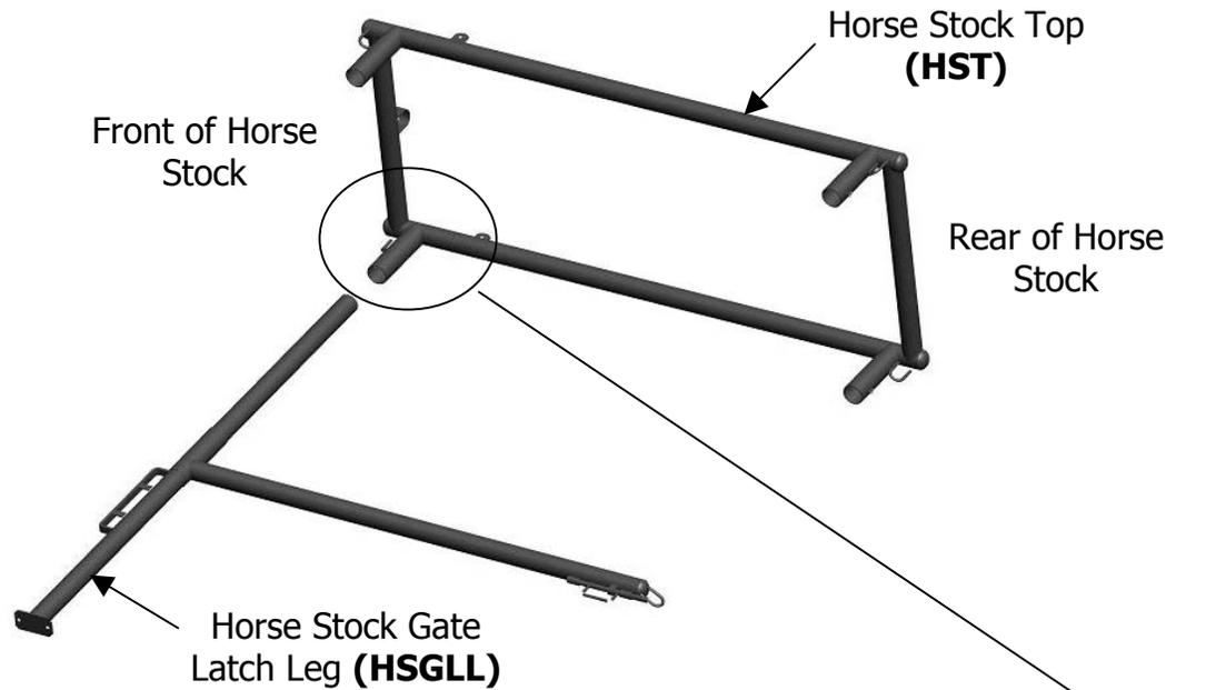
**Step 3:** Lay the (HST) on the ground and turn it up on it's side.
