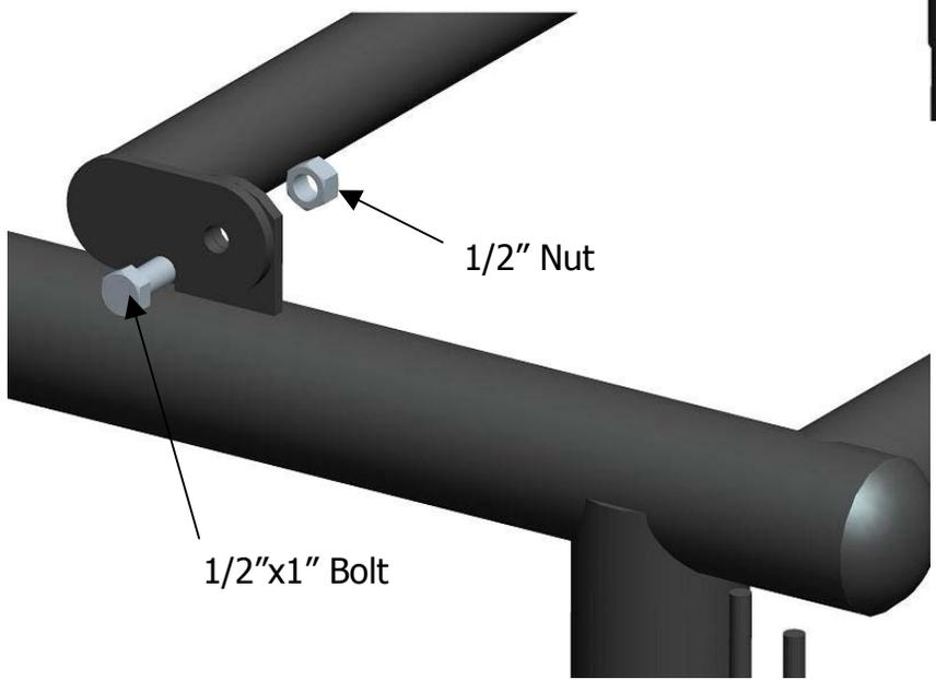
**Step 8:** Insert the (HSTB) through the slot provided on the front of the (HST). Then secure it with the 1/2"x1" bolts & nuts provided. This concludes the Horse Stock Tie Bar installation process.
