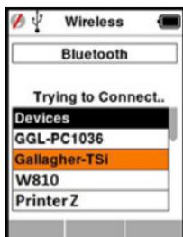
**Note:** The HR5 can be configured to send and/or receive data from other devices via Bluetooth.
