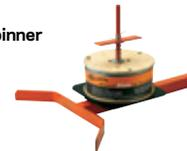
A necessity for building permanent fence. The adjustable break keeps wire from over-spooling and it attaches to a 2" receiver.
