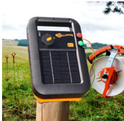
The solar panel charges the battery by converting light directly into electricity. The battery stores this electricity to operate the energizer. This enables the energizer to operate at night or during periods of low sunlight.
