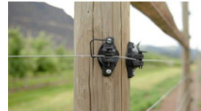
On sharper corners, you may have to fasten the hot wire on the inside of the post to prevent it from touching the post.
