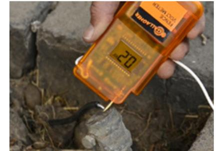
There should be no reading on the Volt Meter; however, up to 200V (0.2kV) is acceptable. If the voltage is higher than this, switch off the Energizer, drive in more ground rods at the recommended spacings and connect them to the existing ground system until the voltage is down to the acceptable level.
