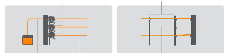
**Power Connectors** are leads that connect a portable fence to an existing permanent electric fence.
