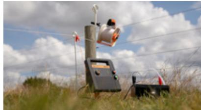
**Solar Energizers** are portable and an excellent choice for temporary fence applications. They are a logical choice for remote areas where there is no 110V outlets. While they have the highest upfront cost per joule, the power to operate them is free as long as they have adequate sunlight.
