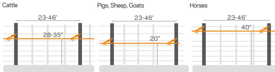
**Offset electric fencing** is an economical and easy to install option if you have an existing or new non-electric fence that you want to protect.
