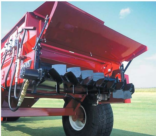
The patent pending Saber Tooth attachment is optional equipment on the Turf Tiger 4300. It is remarkably powerful, yet applies a consistent and uniform spreading pattern that ranges from 8' to 12' wide, depending on the material.
